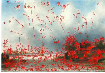
Figure 3.3: Sample DoG Interest Points . Lowe’s DoG detector was used on each image to extract interest points. Each red arrow indicates a feature and orientation, with the length corresponding to the scale of the keypoint.
