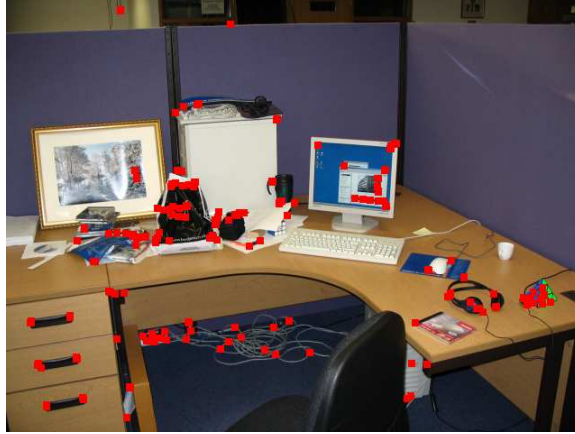
Figure 2.18: Harris Corners This image displays Harris corner detection, with the 200 maximal corners from the image superimposed in red. Notice how the detector fires not only at corners but also at areas of active texture (e.g. the crinkled bag, the tangled wires.)
