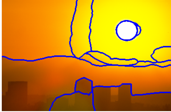
Figure 2.3: Result of Normalized Cuts Segmentation This is an example of a Normalized Cuts segmentation. Note that while it segments out regions which make sense (such as the circle for the sun) it also over-segments smooth areas due to the nature of the stopping condition for the bipartite splitting. Image obtained from Prasad Gabbur.
