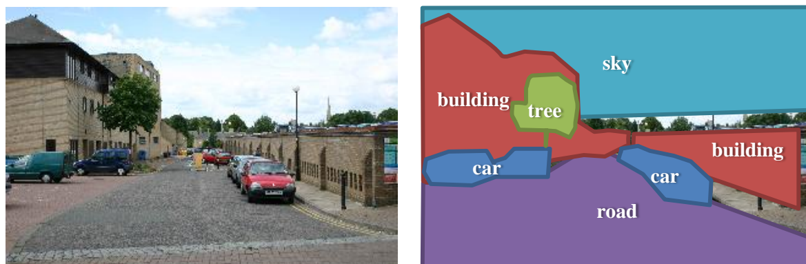
Figure 4.1: Semantic Segmentation . A semantic segmentation of an image is one which groups the pixels together by common semantic meaning. Shown is one such segmentation of an image, using as pixel labels the objects in the scene.
