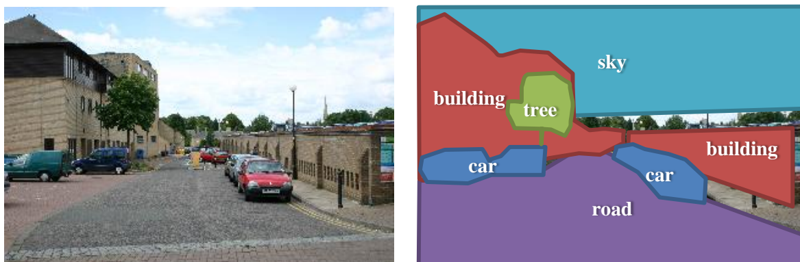
Figure 1.1: An Example Semantic Segmentation. A semantic segmentation of an image is one which groups the pixels together by common semantic meaning. Shown is one such segmentation of an image, using as pixel labels the objects in the scene. This information can be used for automatic image annotation, or for compositional search based upon semantics.
