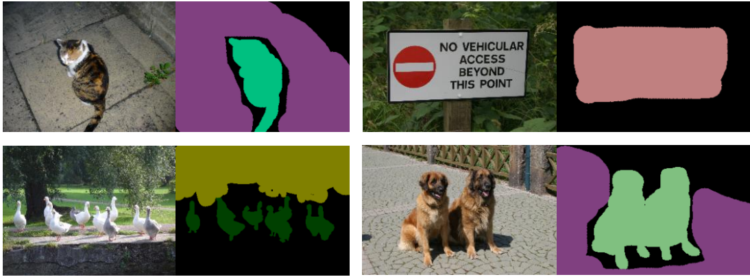
Figure 3.4: Training Data . A tree is trained on ground-truth labeled images like these above, in which a semantic label is associated with each pixel of an image.
